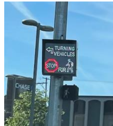
Left Turn Pedestrian Warning Sign
